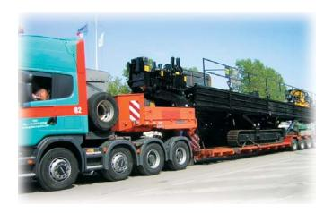
Highway Transport. Although the D200x300 is an overweight load, the unit can be transported any time of day because it's within legal dimensions in the transport mode. The unit features an integral
