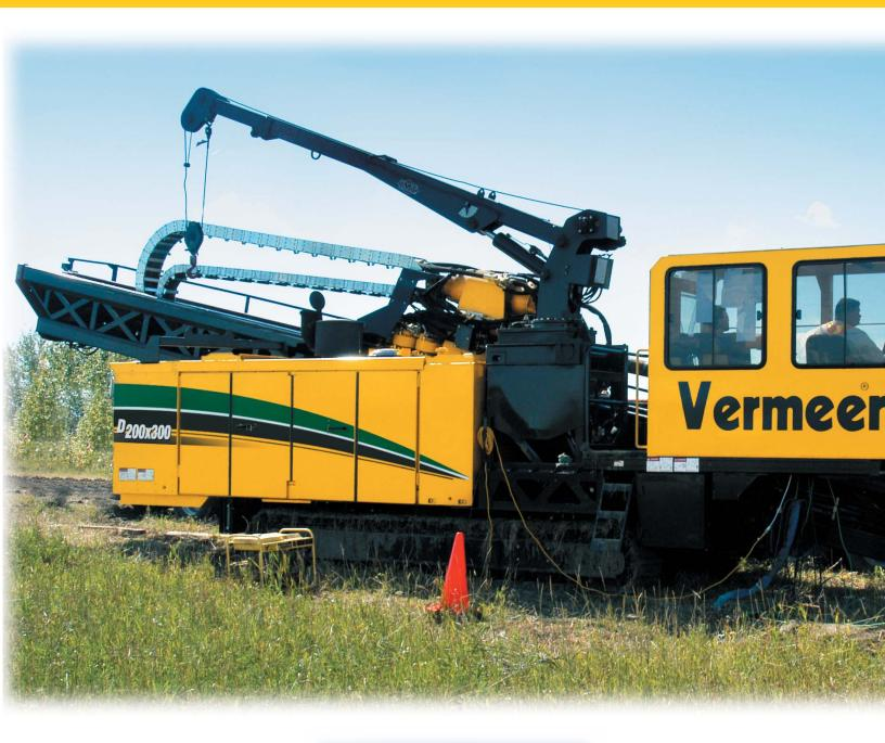
Self Contained Design. The D200x300 offers quick setup time. All components, including the crane and cab, are part of the machine and requires minimal setup time. Only the high pressure fluid line and corresponding electrical line require setup.
