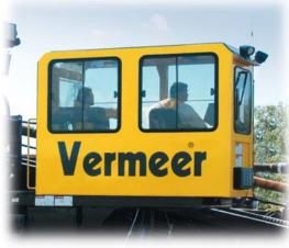
All functions operated from the cab. The D200x300 helps eliminate the need to operate transport, drilling controls, crane and drilling fluids remotely, or to move to a different location on the machine for various functions. This increases manpower efficiency by allowing a single operator to run everything from the operator's station. Also provides room for a second crew member to consult in the drilling operation.
