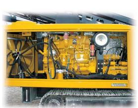
Serviceability. Engine bay doors that fully open on one side of the machine provide easy entry to engine service points, fuel, hydrostatic pumps and filters, and hydraulic diagnostic ports.
