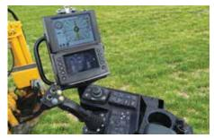
DRILL EFFICIENTLY. The D36x50 Series II features the DigiTrak® Aurora™ full-color touchscreen display, delivering real-time, easy-to-view locate information which can help make a driller's day more productive.
