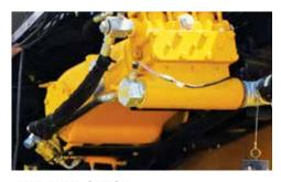
MUD PUMP OPTION. The drill is available with a 50-gpm (189.3 L/min) or 70-gpm (265 L/min) onboard pump, providing higher flow when backreaming, helping increase efficiency.
